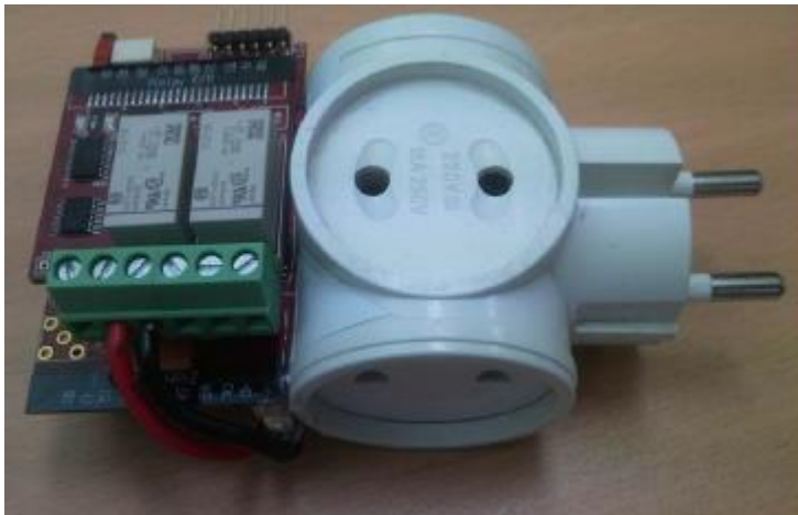
Figure 10: Sensor node with power switching module.
